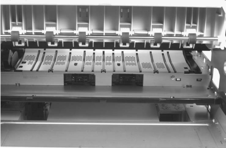
Figure 6-34 Feeder Assembly (2 of 2)
